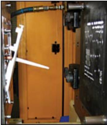
Part stuck on the moving half.
