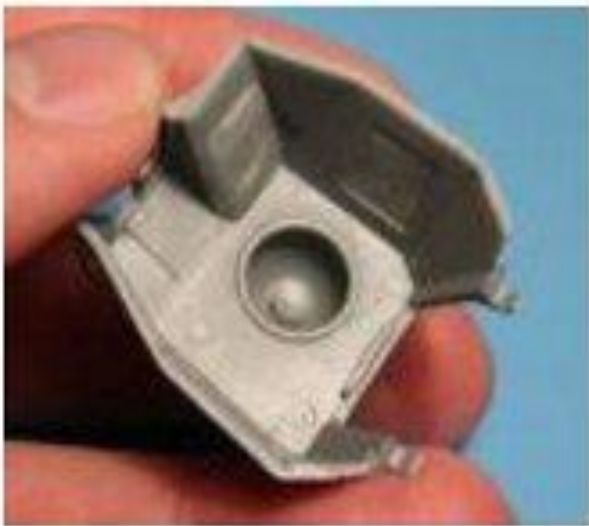
Ejection Pin Marks
